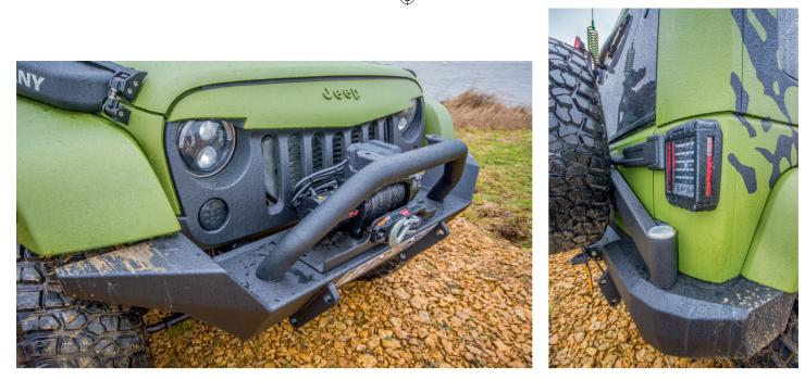
Above left: You'll know about Bestop's canvas products, but the company also makes bumpers. Very serious bumpers at that. This one is home to a Warn Tabor 10-5 winch, which was installed complete with a correctly rated wiring loom – that's the sort of thing that only happens when you get a proper 4x4 specialist to build your truck for you
