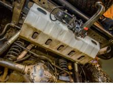
However high you lift your suspension, it doesn't make any difference to the clearance beneath your axles. Hence this AEV rear diff skid plate, which as well as protecting the fragile stuff helps lift it over any obstacles that pop up out of the ground thinking evil thoughts
