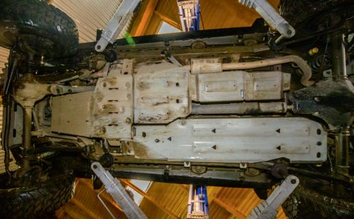
Above: Rival's 6mm aluminium underbody protection plates are still relatively new to the UK, but they're quickly becoming part and parcel of top-end builds. And quite right too: protecting your investment is simple common sense, after all. The Russian company makes a comprehensive set of plates that go together to turn the Jeep's underside into something resembling the hull of a barge; about the only things here that don't have plates protecting them are the plates themselves
