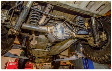
On pretty much anything that's not a Rubicon, you'd be looking at the pictures above while we went on about the trick diffs and heavy-duty halfshafts inside the axles. No need to here, though. This is a truck that came out of the factory on Dana 44 axles with Jeep's own Tru-Lock diffs - you'd need to be fitting a truly enormous set of tyres before you had to start thinking about strengthening them further
