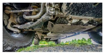
Rival's underbody protection kits have become increasingly popular over the last couple of years or so, especially on pick-up builds, and Andy's Ranger wears a full set of 6mm aluminium plates stretching just about its entire length. There's another kind of protection going on under here, too - to help keep it strong and sturdy in the face of a tough life, the chassis received the full Dinitrol wax treatment
