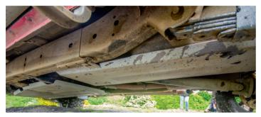
Underneath, a full set of 6mm aluminium bash plates protects the delicate bits from inevitable comingstogether with terra firma – and also acts like a giant ski for when the sort of breakover angle endemic to longwheelbase vehicles like the Ranger threatens to become its Achilles' heel
