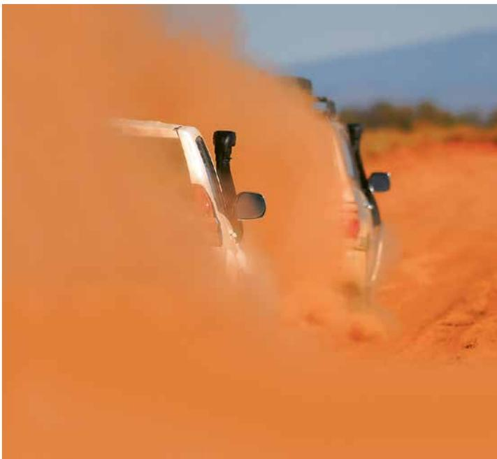
Created to protect 4WD engines from the hazards of dust and water ingestion commonly encountered in off road driving, Safari snorkels relocate your air intake point from the relatively low and vulnerable position under the bonnet to a higher and safer location, where a constant source of cool, clean, dry air is available.
