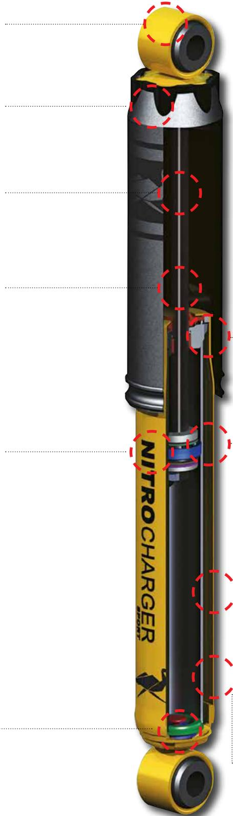
The rod guide has been engineered with a less restrictive design and open apertures to ensure a more uniform oil flow through the disc stacks. This improves control over a higher temperature range – as the shock absorber heats up, oil flow over the valving remains stable, giving dependable, fade free damping. A Teflon infused bronze slip ring has also been incorporated into the rod guide to ensure tight manufacturing tolerances are maintained.
